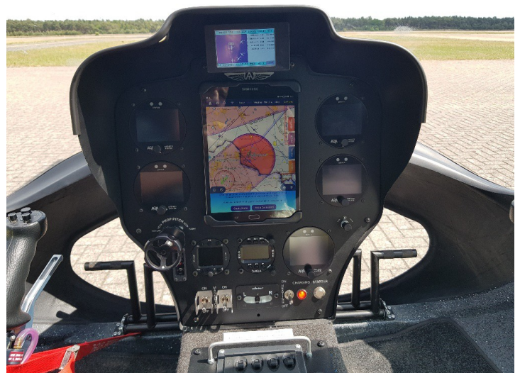
The RTIS ADSB system installed in a Trendak Tercel Gyro.
